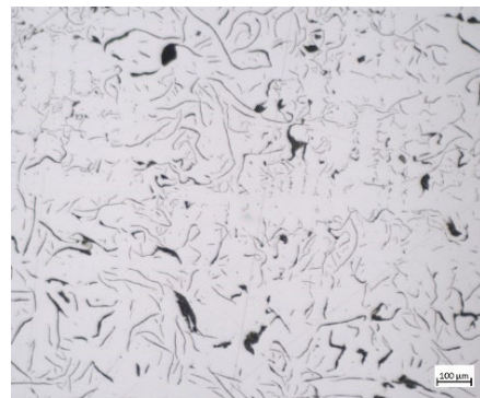
Figure 2. A micrograph of unetched gray iron.
